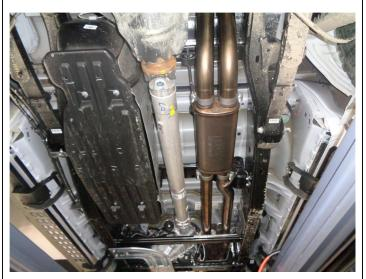
**Step 6.** Install the Muffler Assembly by attaching the the inlet nipples to the outlets of both Inlet Pipe Assemblies. Loosely secure using the supplied clamps. Engage the welded hanger to the rubber insulator.
