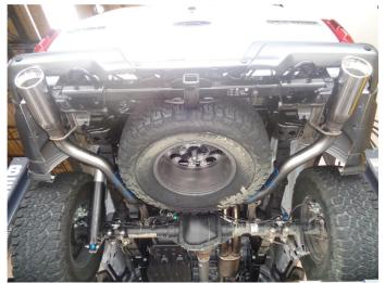
**Step 8.** Lastly loosely attach both Tail Pipe Assemblies to the Over Axles Pipes using the supplied clamps. Engage all welded hangers to the rubber insulators.
