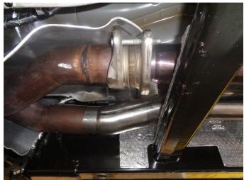
Step 4. - NOTICE - this exhaust kit works with both the SuperCrew and SuperCab models. The SuperCrew has adittional parts. Begin the installation by slipping the inlet of the P/S Inlet Pipe Assembly into the OEM band clamp. On the SuperCab model engage the welded hanger into the rubber insulator. Next bolt the D/S Inlet Pipe assembly to the OEM flange junction using the supplied nuts. All clamps and fasteners are to remain loose until final installation.
