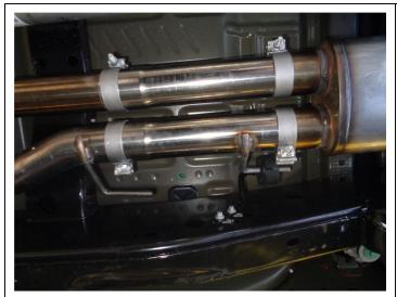
**Step 5.** FOR THE SUPERCREW ONLY, install both extension pipes into the resonator outlets and engage the hanger into the rubber insulator.
