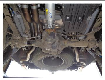
**Step 7.** Loosely attach both Over Axle Pipes to the Muffler Assembly outlet nipples using the supplied clamps.
