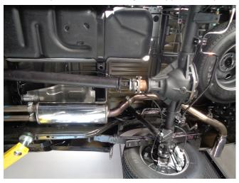
Step 4: Loosely attach the Muffler Assembly to the two Extension Pipes using the supplied clamp and engaging the welded hanger to the rubber insulator. Install the Tail Pipe Assembly the same way.
