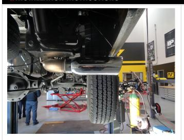
Step 5: Once a final position has been chosen for the new exhaust system, evenly tiligten all clamps from front to rear using the torque specifications on page one of these instructions. Inspect all fasteners after 25-50 miles for operation and re-tighten if necessary.
