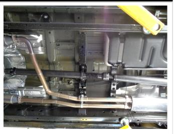
Step 3: Next loosely fasten both Extension Pipes to the Inlet Pipe Assemblies using the supplied clamps.
